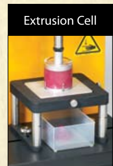
Extrusion cell fixture allows backward or forward extrusion. Ideal for pie filling, toppings and more.
