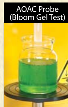
An industry approved probe and sample jar provides consistent gelatin bloom tests.
